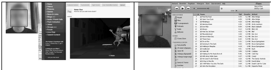
Fig. 21. Using a face detector and a speech recognizer in combination with screen poking to control applications. Horizontal face coordinates control the online game (left), while vertical face movements and speech control the iTunes software (right).
